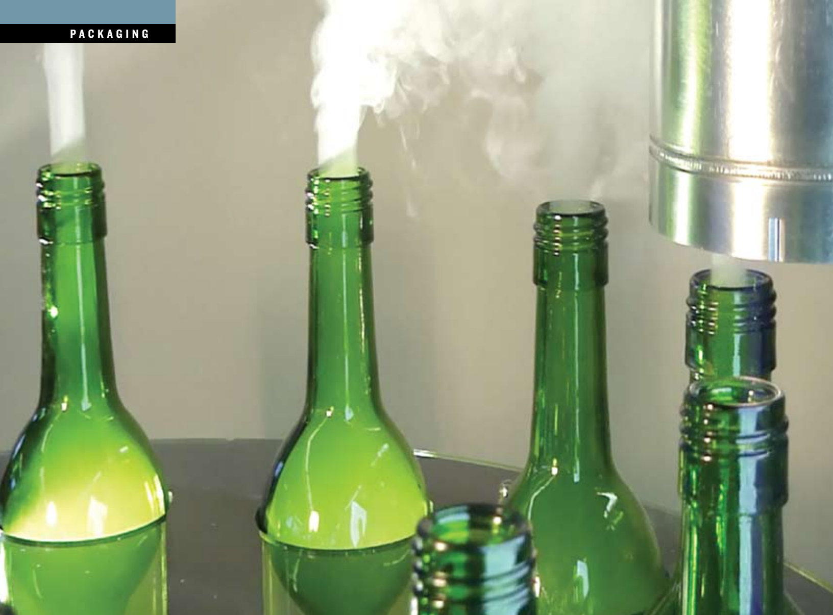
John Davis says the Nitrodose Easy Dose liquid nitrogen injection system (above) fits easily into AT Mobile Bottling Line's compact setup.
